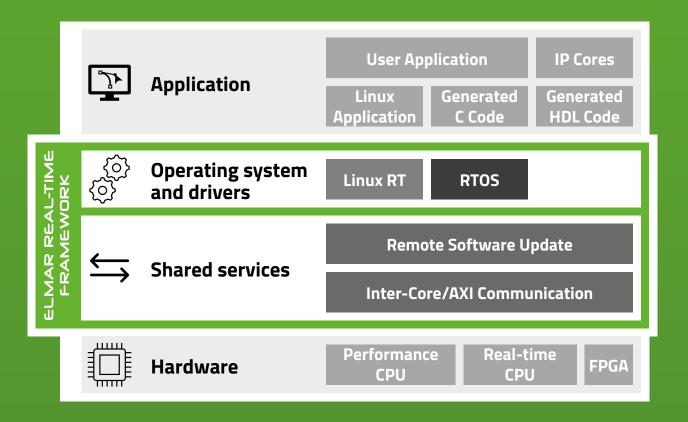
By applying our kernel patch, which has been specially developed for this platform,we can guarantee a stable 10 kHz frequency on the real-time cores. This is measured using a complex industrial Simulink<sup>®</sup> control algorithm.
